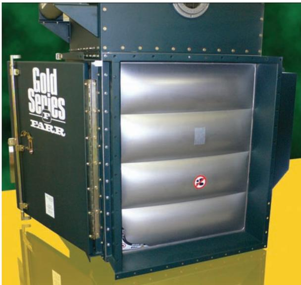
designed explosion vent functions as a weak element in the equipment's pressure envelope, relieving internal combustion pressure (back pressure) to keep the collector from blowing up into pieces. The vent's function is illustrated in Figure 2, a series of photos showing a staged deflagration in a cartridge dust collector equipped with an explosion vent. Typically, the collector is located outside and de-
